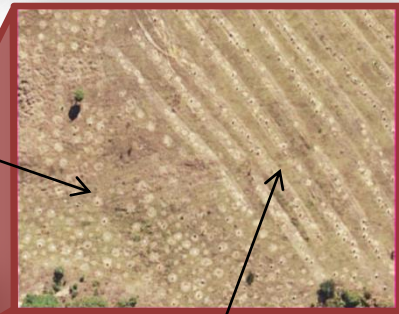
Ground preparation for "contour" planting areas including ripping and spraying lines on the contour.
